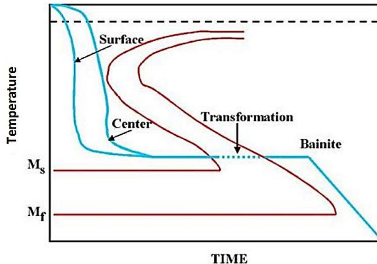
**Figure 6.** Cooling diagram of austempering process [10].
