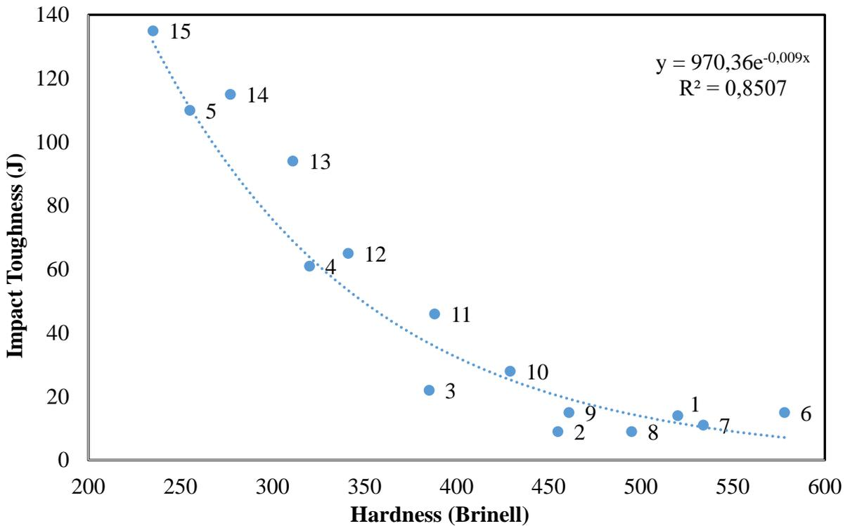
Figure 15. Hardness vs Toughness graph of the specimens [15].
