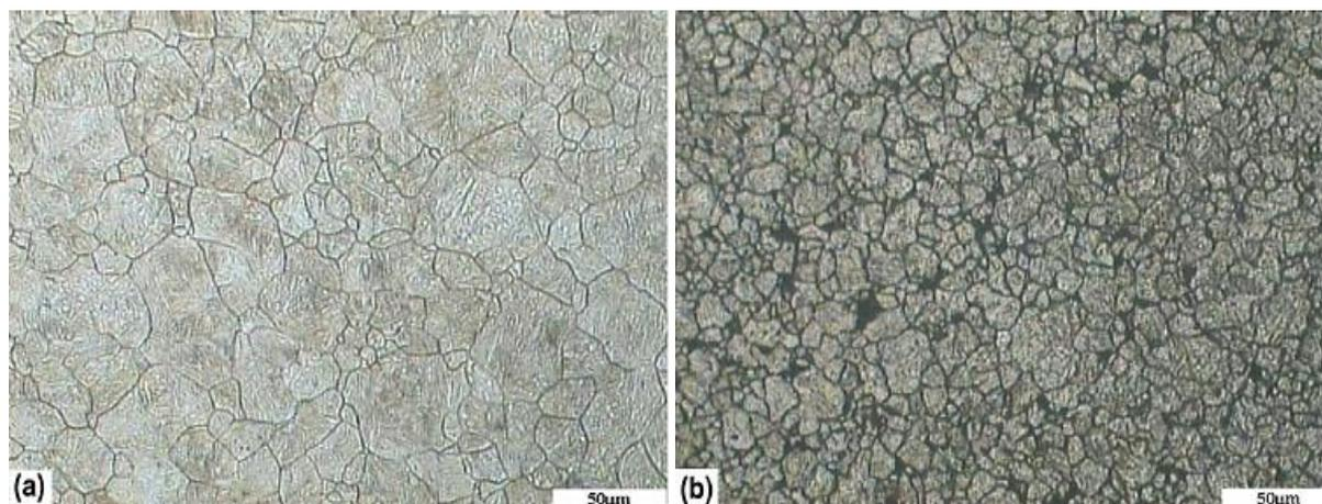
**Figure 10.** The prior austenite grain boundary networks developed from the specimens treated as: (a) CQT and (b) DQT heat treatments [12].
