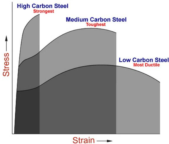
**Figure 1.** Typical Stress - Strain curves for different material compositions [1].
