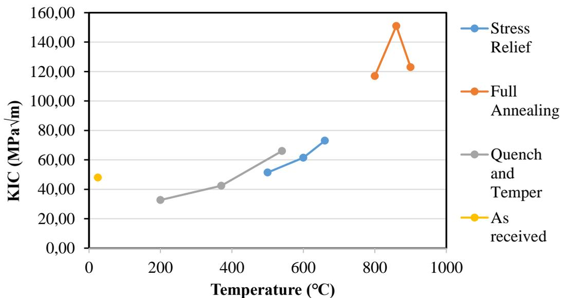
**Figure 13.** Fracture Toughness-Temperature graph of heat-treated samples [14].
