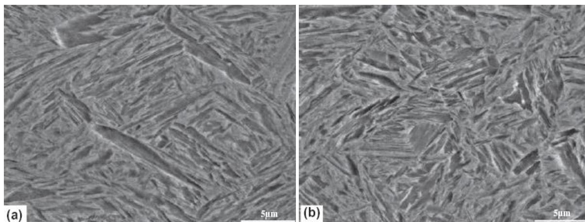
**Figure 11.** SEM micrographs showing the martensitic packets in the heat-treated specimens: (a) CQT and (b) DQT conditions [12].
