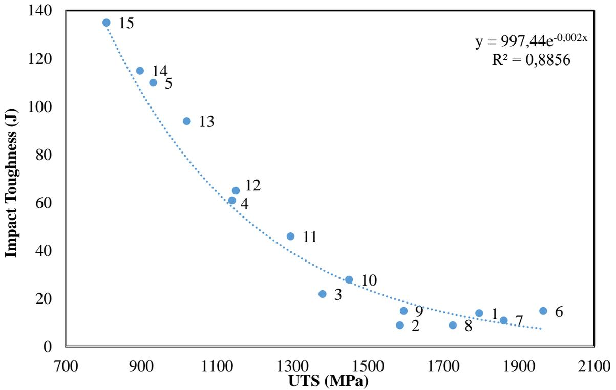
Figure 14. UTS vs Impact Toughness graph of the specimens [15].
