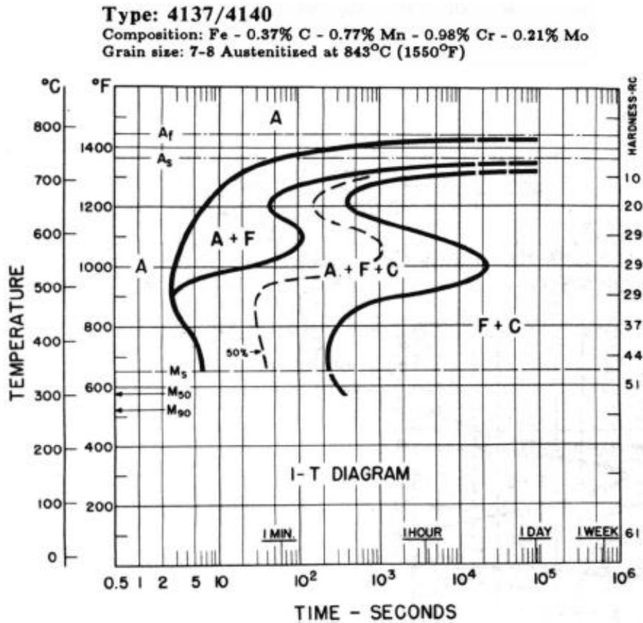
**Figure 2.** Isothermal Time-Temperature-Transformation (TTT) curve for AISI 4140 low alloy steel [6].
