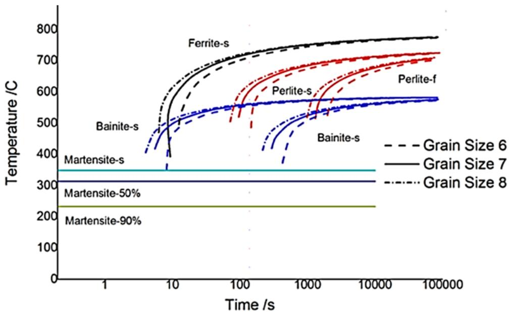
**Figure 3.** 4140 CCT diagram based on different grain sizes [5].
