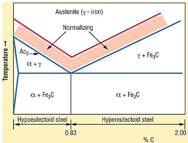
**Figure 7.** Normalizing temperature range superimposed on the standard phase diagram of steels [11].
