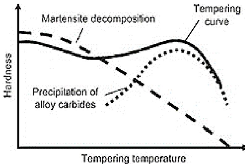
**Figure 4.** Effect of tempering temperature on secondary hardening [9].
