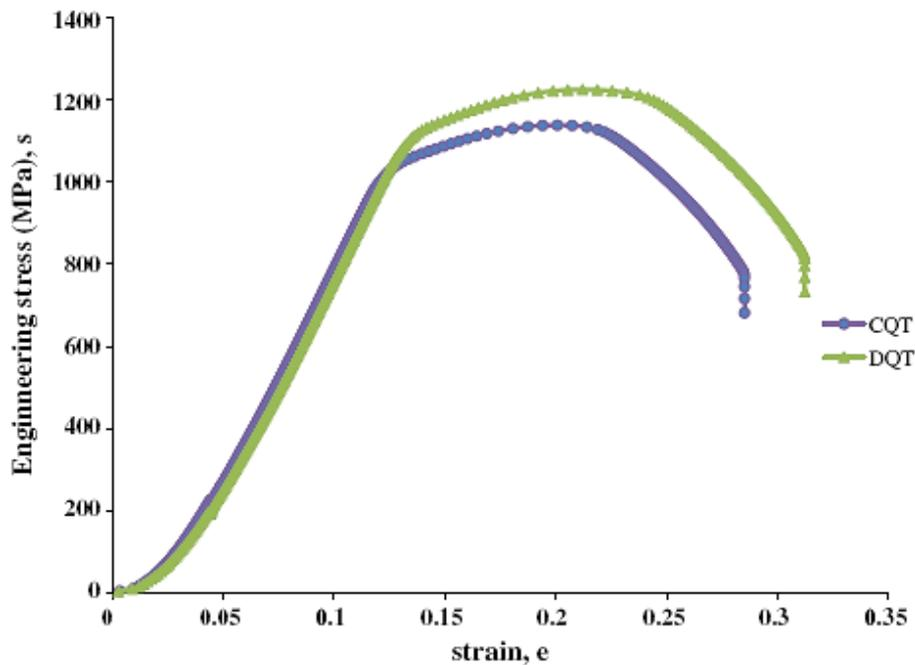
**Figure 9.** The engineering stress–strain behavior of CQT and DQT specimens [12].
