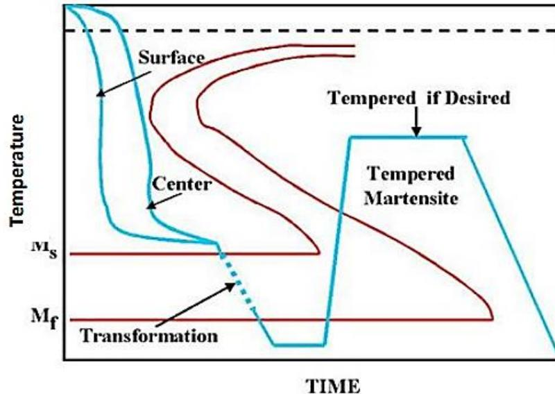
**Figure 5.** Cooling diagram of martempering process [10].
