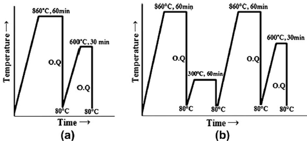
**Figure 8:** Time-Temperature lines of heat treatment processes: (a) CQT and (b) DQT [12].
