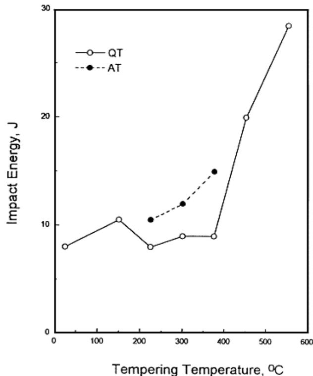
**Figure 12.** Charpy impact values of 4140 specimens according to tempering temperature [13].
