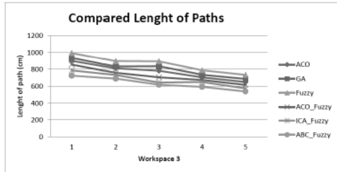
Fig. 5 Comparison of path length in quite complicated workspace by the Purposed Hybrid algorithms and ABC-Fuzzy.
