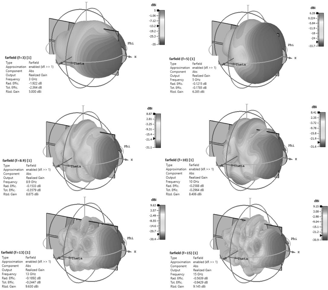
Figure 5: Simulated radiation pattern of the antenna at 3 GHz, 5 GHz, 8.9 GHz, 10GHz, 13 GHz and 15 GHz.
