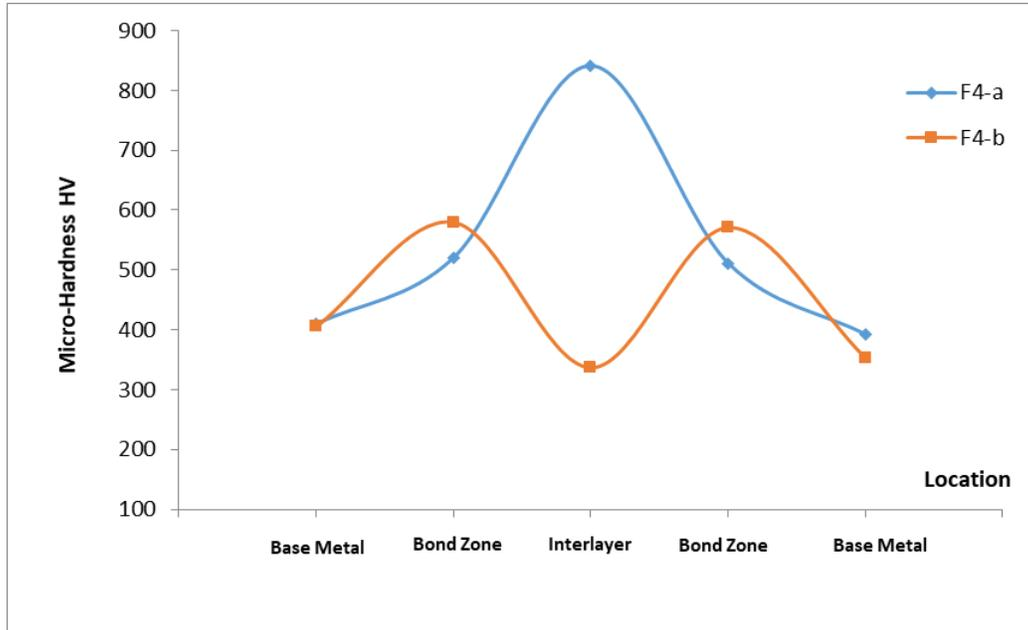
**Figure 4.** Vickers Micro-Hardness profile across joint-line of IN 738LC brazed by F4-a and F4-b.
