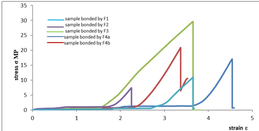
**Figure 2.** Stress-strain curves during shear test on tensile machine for samples bonded by F1, F2, F3, F4a, and F4b.
