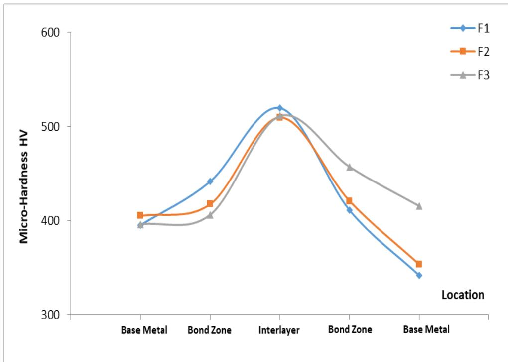
**Figure 3.** Vickers Micro-Hardness profile across joint-line of IN 738LC brazed by F1, F2, F3.
