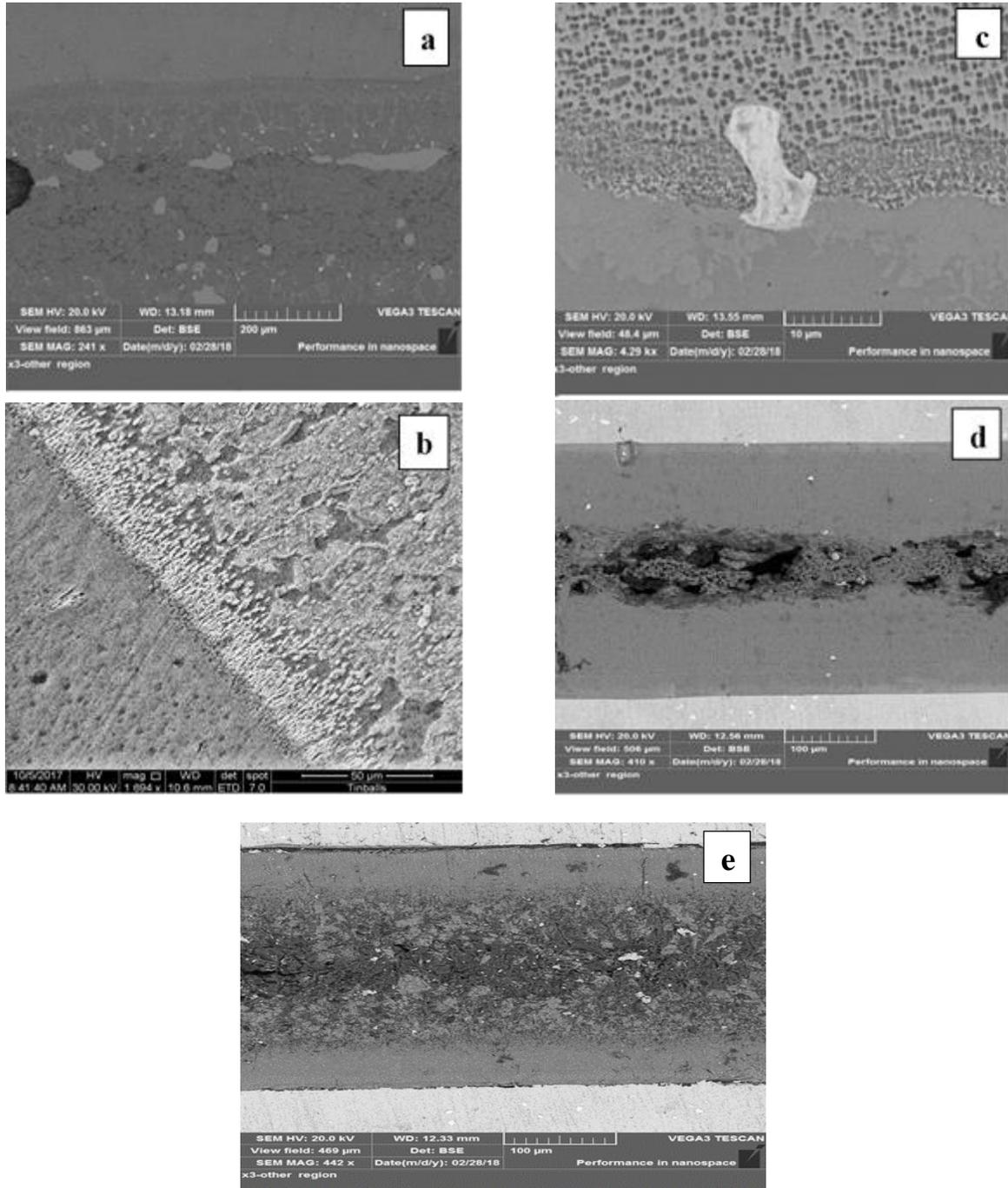
**Figure 1.** SEM image of microstructure for sample bonded by a) F1 (241x), b) F2(4.29kx), c) F3(1684x), d) F4 (410x) and e) F5(442x).
