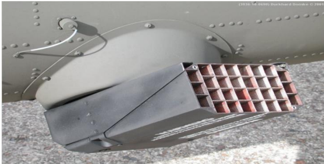
Fig. 3 Countermeasure Dispenser System integrated in a Helicopter (close view)
