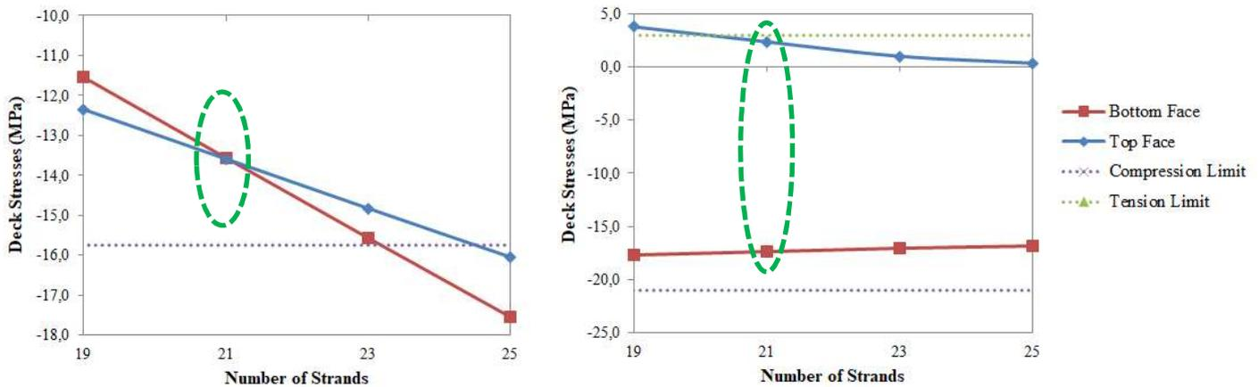
Figure 10. Deck Type 2, Stresses vs. Strands Graph (First Stage & Service Stage, Respectively)
