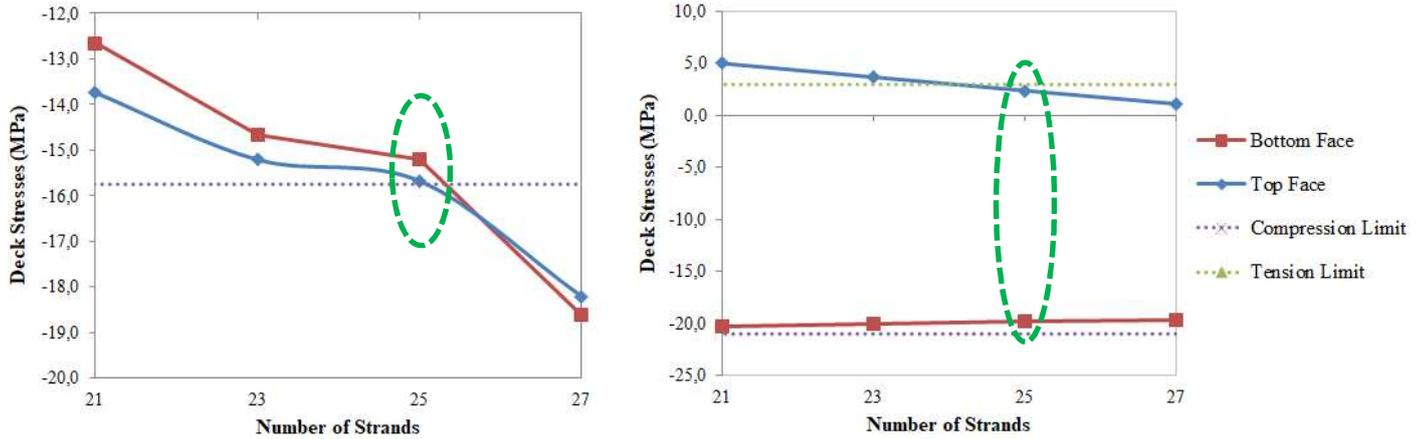
Figure 11. Deck Type 3, Stresses vs. Strands Graph (First Stage & Service Stage, Respectively)
