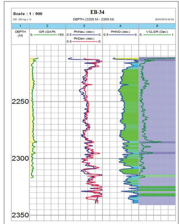
**Figure 5.** Corrected well log data for well EB-34.
