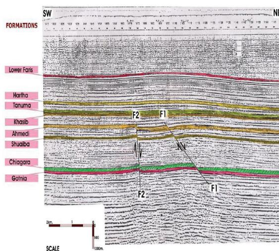
**Figure 2.** Seismic cross section with hydrocarbon source, reservoir, and seal rock units in East Baghdad Oil Field. Double line arrows indicate directions of migration pathways, while F1 and F2 are normal faults (modified after Al-Ameri, 2011).
