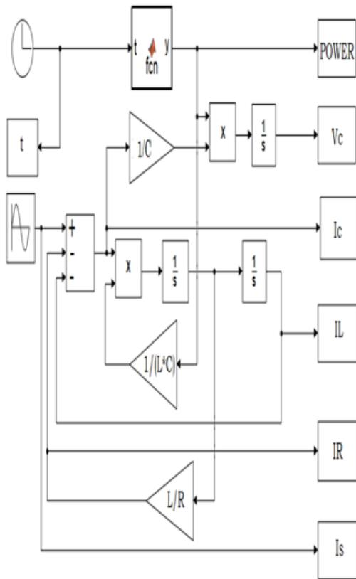
**Figure 4.** Simulink block diagram of the parallel circuit excited with a sinusoidal current source.
