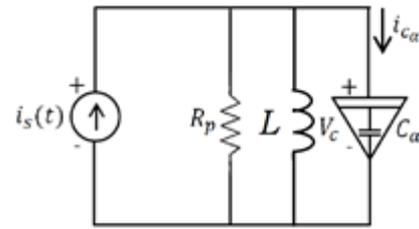
Figure 1: The parallel circuit with a CFD capacitor.
