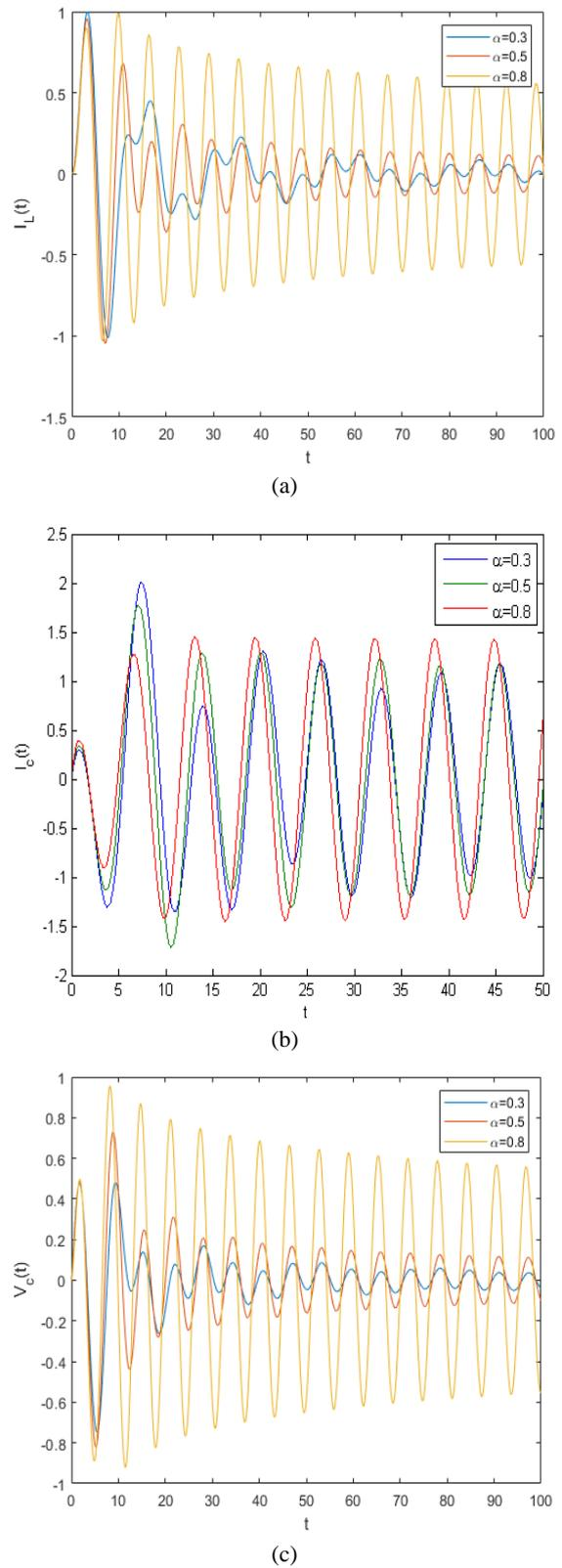
**Figure 5.** a) The inductor current, b) the CFD Capacitor current and c) the CFD Capacitor voltage vs time when the parallel circuit is fed by the sinusoidal current source simulated for three different alpha values.
