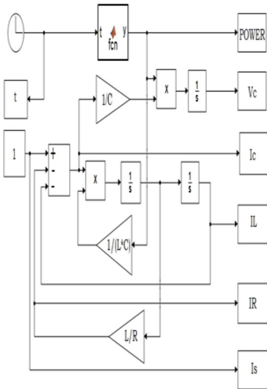
**Figure 2.** Simulink block diagram of the parallel circuit excited with a constant current source.
