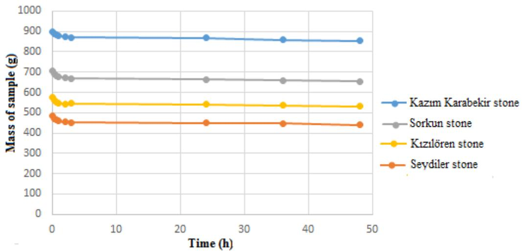
Fig. 4. Mass change of stones according to time in drying test
