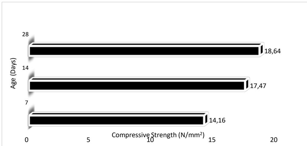
**Figure 4.** Compressive strength of 3.35-10mm coarse aggregate.
