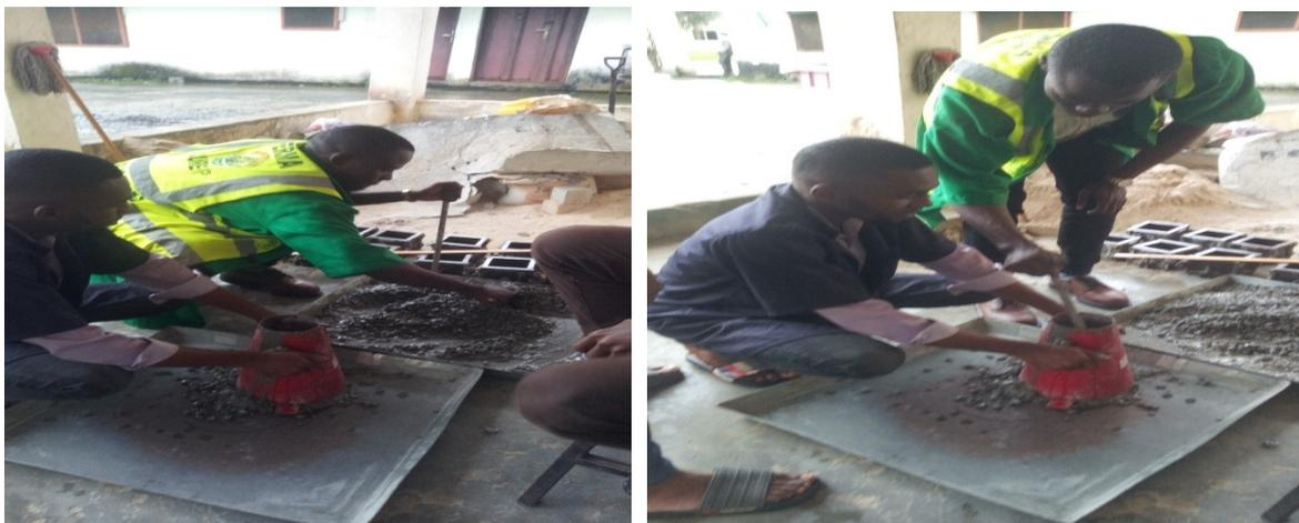
Figure 1. Slump test Experiment.
