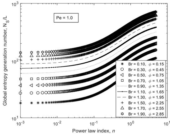
**Figure 17.** Global entropy generation number per unit length as a function of  $n$  for various values of  $Br$  and  $\phi$  at  $Pe = 1.0$ .
