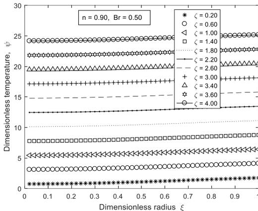
**Figure 5.** Variation of dimensionless temperature with an axial distance at constant  $n$  and  $Br$ .
