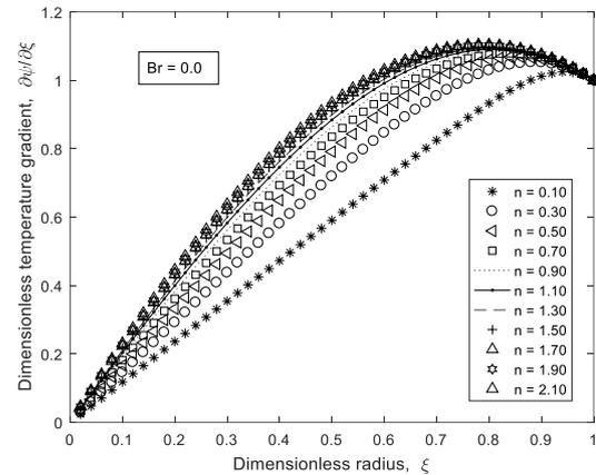
**Figure 6.** Dimensionless temperature gradient as a function of  $\xi$  for various values of  $n$  at  $Br = 0$
