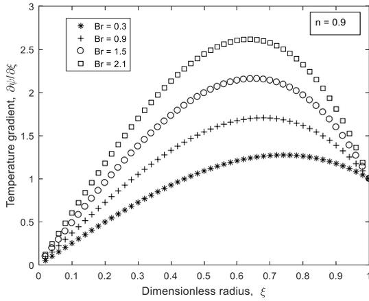
**Figure 7.** Temperature gradient as function of  $\xi$  for various values of  $Br$  at  $n = 0.90$ .
