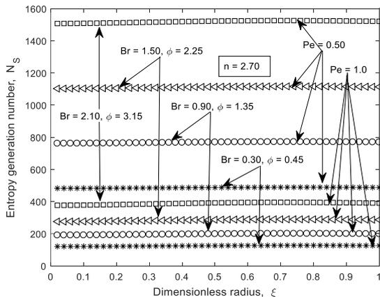
**Figure 15.** Entropy generation number as function of  $\xi$  for various values of  $Br$  and  $\phi$  at  $Pe = 0.5-1.0$  and  $n = 2.70$ .
