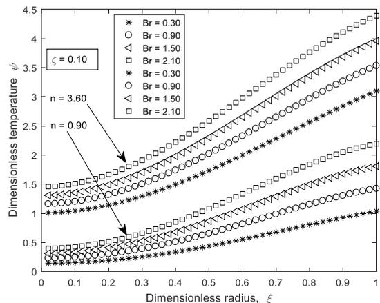
**Figure 4.** Dimensionless temperature as a function of  $\xi$  for various values of  $Br$  and  $n$  at  $\zeta=0.10$ .
