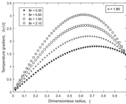
**Figure 8.** Temperature gradient as function of  $\xi$  for various values of  $Br$  at  $n = 1.80$ .
