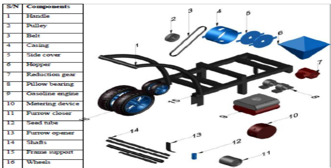
**Fig. 1.** The exploded view of a maize planter showing the major components.
