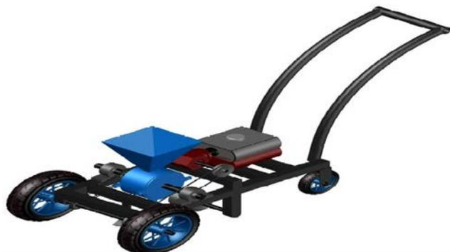
**Fig. 2.** Isometric view of the maize planter.
