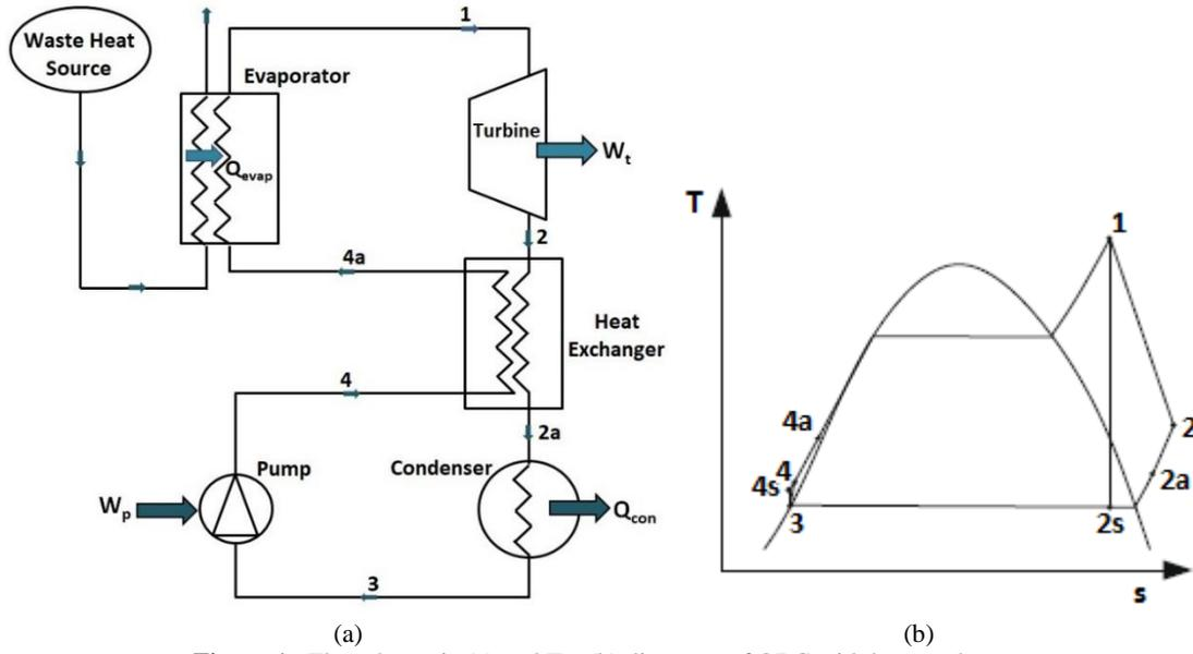
Figure 1. The schematic (a) and T-s (b) diagrams of ORC with heat exchanger
