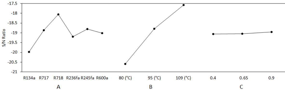
**Figure 12.** The effects of each design parameter on thermal efficiency
