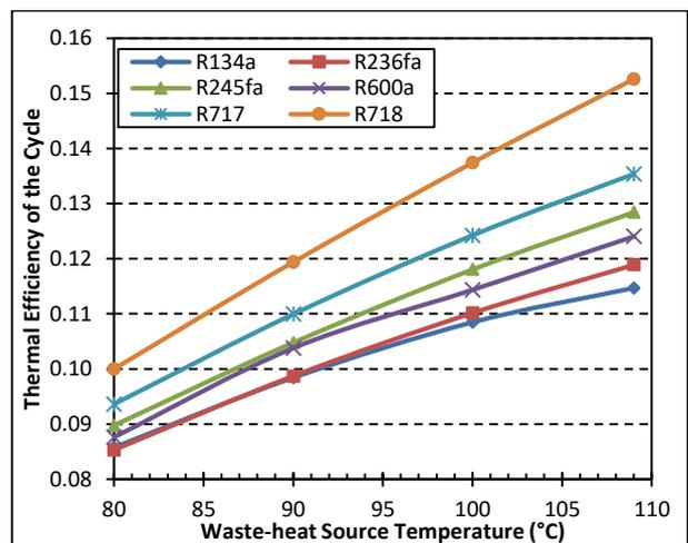
**Figure 6.** The change of the thermal efficiency of the cycle depending on waste-heat source temperature
