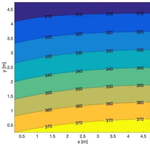
**Figure 10.** Temperature distribution for the square plate
