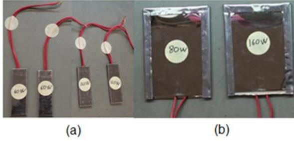
Figure 5. (a) Partial heaters; (b) whole heaters
