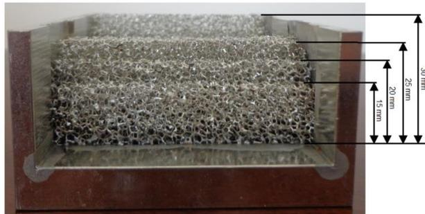
**Figure 4.** Porous layers of foam embedded heat sink
