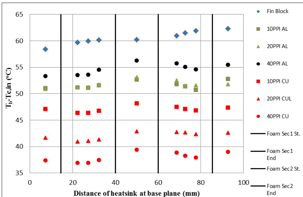
**Figure 13.** The variation of the base plane temperatures as a function of the distance at 160 W heater
