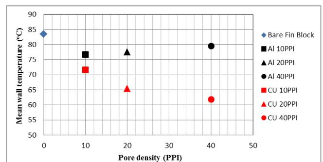
**Figure 10.** Mean wall temperature as a function of pore density at 160 W heater and 6 m/s frontal air velocity
