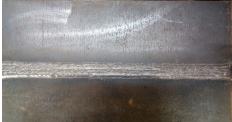
Figure 1. Welded S355JR and weld seam.
