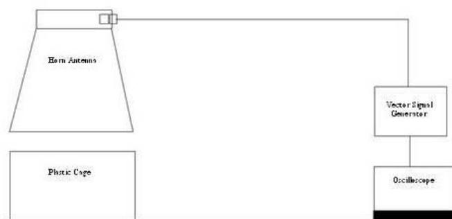
**Figure 2.** ELF Radiation exposure system<sup>23</sup>
