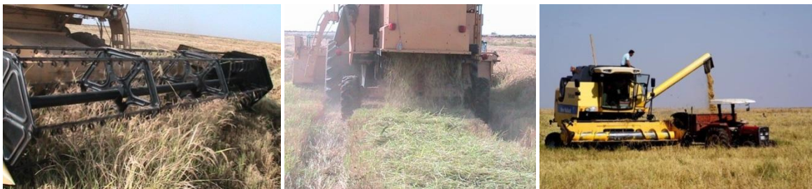
Figure 3. Directly paddy harvesting by self-propelled combine- harvester.
