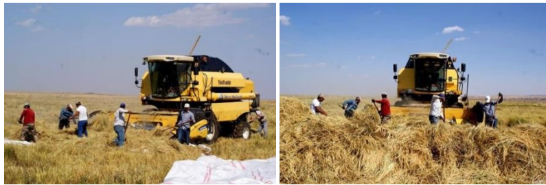
Figure 2. Feeding plant materials to header of stationary combine for threshing.
