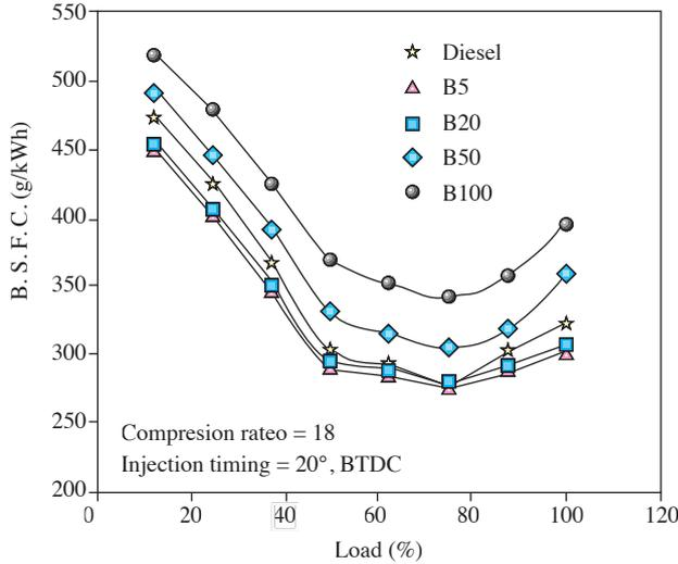
**Figure 8.** Variation in brake specific fuel consumption.
