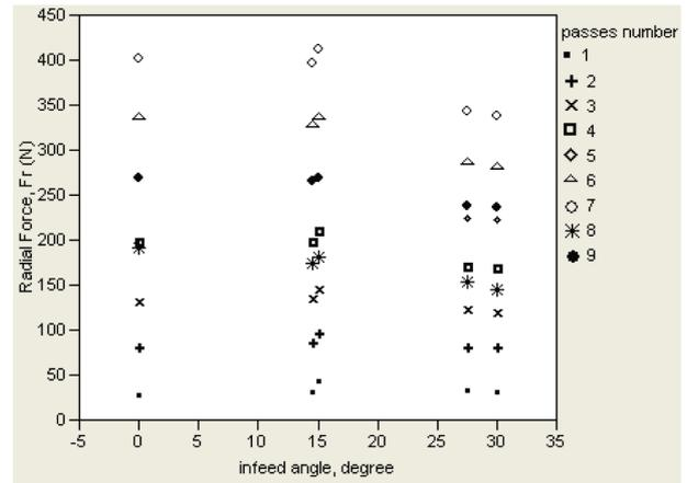
Figure 8. Radial force ( $F_r$ ) change due to different infeed angles.
