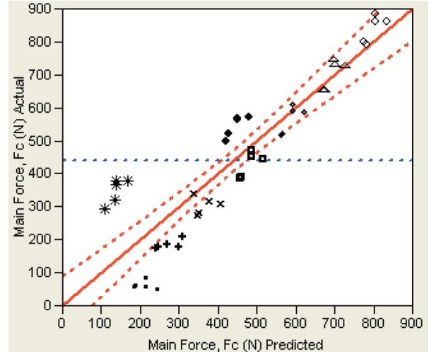
**Figure 3.** The plot of actual main cutting forces versus predicted main cutting forces.
