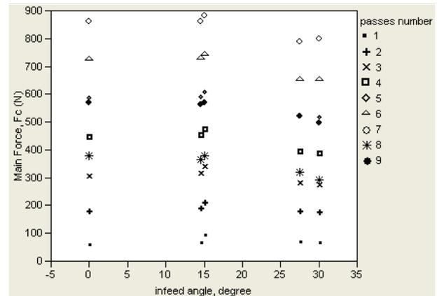
**Figure 4.** Main cutting force (F<sub>c</sub>) change due to different infeed angles.
