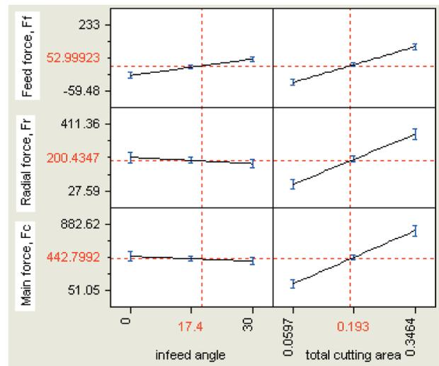
Figure 9. The main effects of infeed angle and total cutting area on cutting forces.
