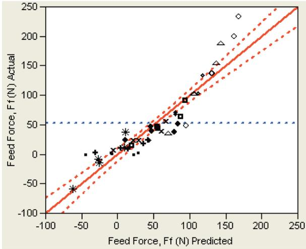
**Figure 5.** The plot of actual feed forces versus predicted feed forces.
