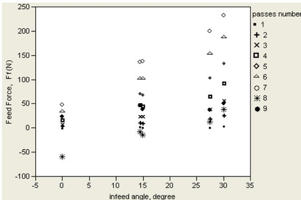
**Figure 6.** Feed force ( $F_f$ ) change due to different infeed angles.
