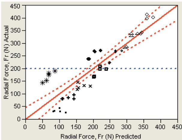
Figure 7. The plot of actual radial forces versus predicted radial forces.
