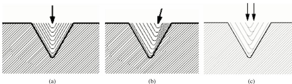
**Figure 2.** Infeed methods. (a) Radial infeed, (b) Flank infeed, (c) Alternating flank infeed (Metalworking, 2005).
