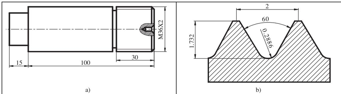
**Figure 1.** a) Shape of the workpiece specimen. b) Thread dimensions.
