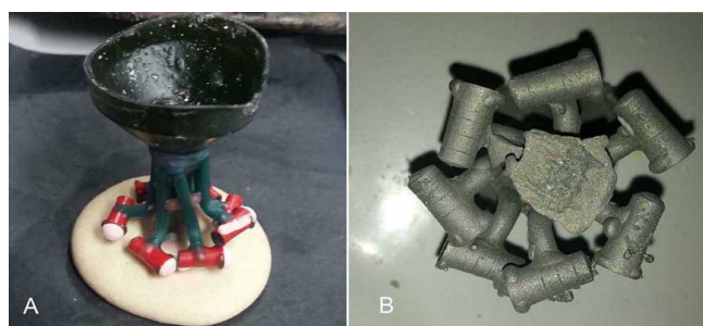
Figure 2. Production of cobalt–chromium alloy crowns.
