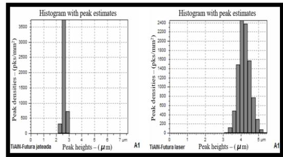
**Figure 16.** Jetting and laser blasting substrate scanned area (A1) and peak density estimate for TiAlN-Futura coatings
