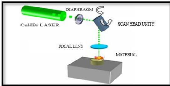
**Figure 2.** Laser texturization experimental assembly scheme [11]
