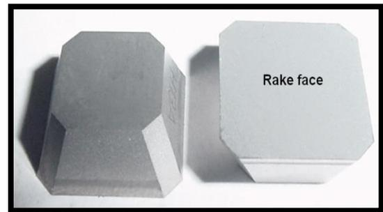
**Figure 1.** Hard metal inserts used for texturization.
