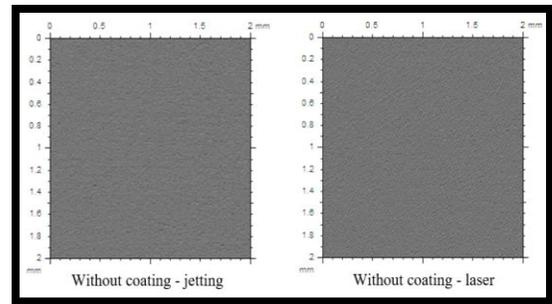
**Figure 21.** Jetting and laser blasting 3D profilometry of surface texture for substrates without coating
