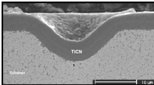
**Figure 4.** Crater formed in a hard metal tool when textured by laser and subsequently coated with TiCN [12]
