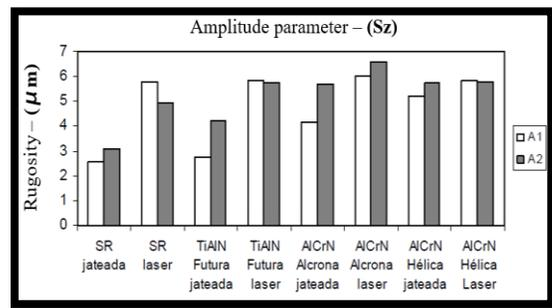
**Figure 10.** Jetting and laser blasting scanned areas (A1, A2) with the height average of ten largest peak-valley distances (Sz) of the textured tools
