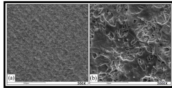
**Figure 7.** (a) SEM of hard metal substrate with laser and without coating deposition. (a) 200x; (b) 2000x
