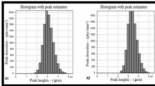
**Figure 15.** Laser blasting scanned areas (A1, A2) with the estimate peak density of textured substrate without coating
