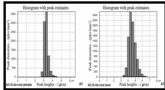
**Figure 17.** Jetting and laser blasting substrate scanned area (A1) and peak density estimate for AlCrN-Alcrona coating
