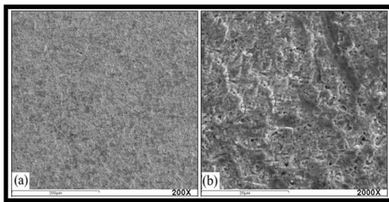
**Figure 6.** (a) SEM of hard metal substrate with jetting and without coating deposition. 200x; (b) 2000x
