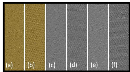
**Figure 22.** 3D profilometry of the surface texture of coated substrates. Jetting: (a) A1CrN-Hélica jateada, (c) A1CrN-Alcrona, (e) TiAlN-Futura; – Laser: (b) A1CrN-Hélica, (d) A1CrN-Alcrona, (f) TiAlN-Futura
