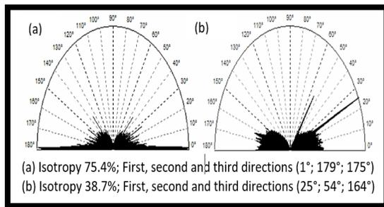
**Figure 23.** Polar graph texture indicator for (a) SR-Jetting and (b) SR-Laser substrates
