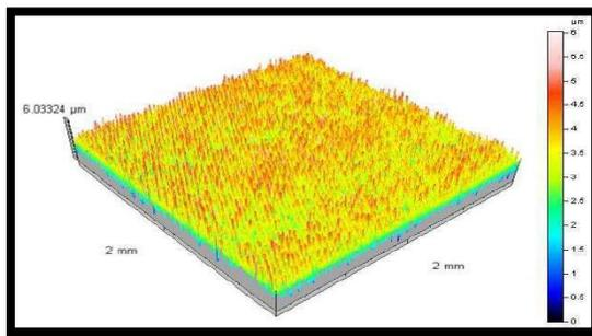
**Figure 20.** Laser blasting 3D roughness profilometry of the substrate without coating
