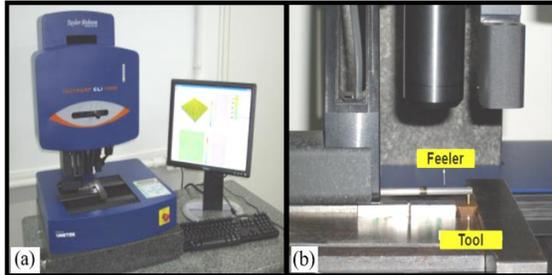
**Figure 5.** (a) 3D profilometer; (b) tool and feeder output surface in detail
