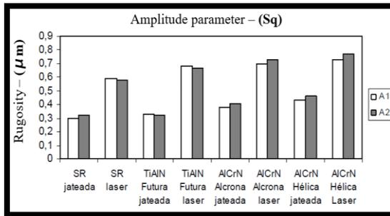
**Figure 9.** Jetting and laser blasting scanned areas (A1, A2) and the mean square surface deviation (Sq) of the textured tools
