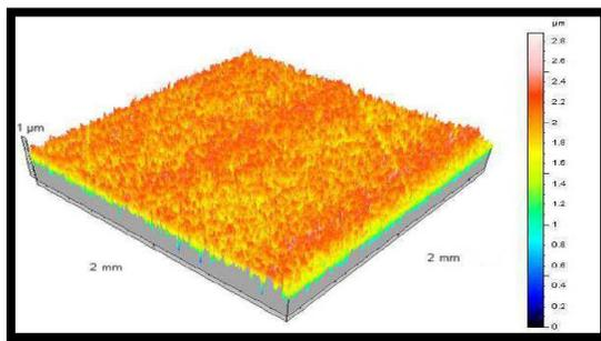
**Figure 19.** Jetting modified 3D roughness profilometry of the substrate without coating
