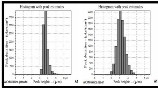
**Figure 18.** Jetting and laser blasting substrate scanned area (A1) and peak density estimate for A1CrN-Hélica coating
