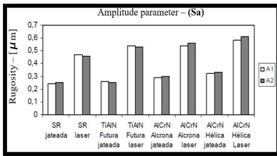
**Figure 8.** Jetting and laser blasting scanned areas (A1, A2) and the arithmetic average surface deviation (Sa) of the textured tools
