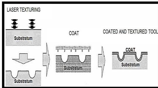
**Figure 3.** Laser texturization steps for a hard metal substrate [12]
