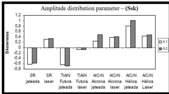
**Figure 12.** Jetting and laser blasting scanned areas (A1, A2) with skewness (Ssk) of the textured tools
