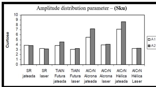
**Figure 13.** Jetting and laser blasting scanned areas (A1, A2) with Curthose (Sku) of the textured tools
