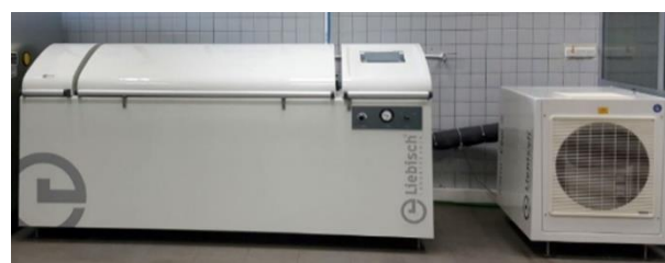
Figure 2 Test equipments; (a) Axial load fatigue and (b) salt spray testing chamber.
