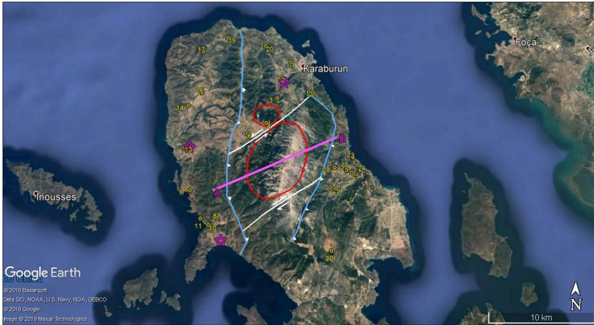
Figure 14. Potential oil and/or gas traps (red polygons) in the study area. Yellow circles: the water samples containing mature petroleum hydrocarbons, pink stars: formerly mercury mines, white lines: strike-slip faults, blue lines: thrust faults. A-B line: taken profile to determine the depth of structure (see Figure 11).
