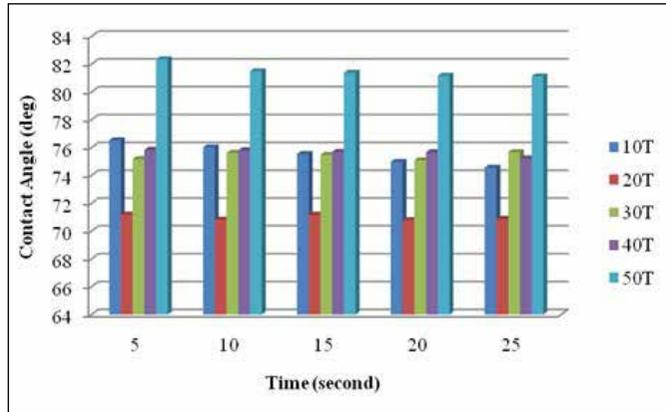
**Figure 3.** Effect of the loading flour on the wettability values of the heat treated wood flour SMA composites (**T**: treated wood SMA composite).
