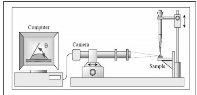
**Figure 1.** Scheme of contact angle determination device.
