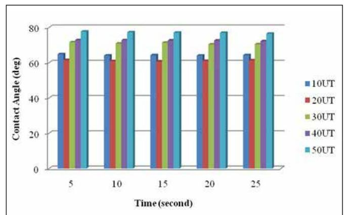
**Figure 2.** Effect of the wood flour loading on the wettability values of the wood flour SMA composites (UT: untreated wood SMA composite).
