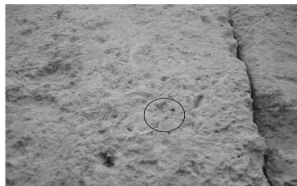
Figure 10. Caloplaca flavescens (Huds.), on calcarenite stone examined after 3 months of exposure to the atmosphere action.
