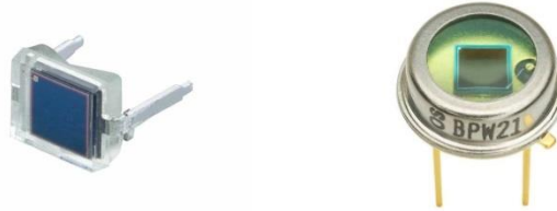
Figure 3. BPW34 and BPW21 silicon photodiode.
