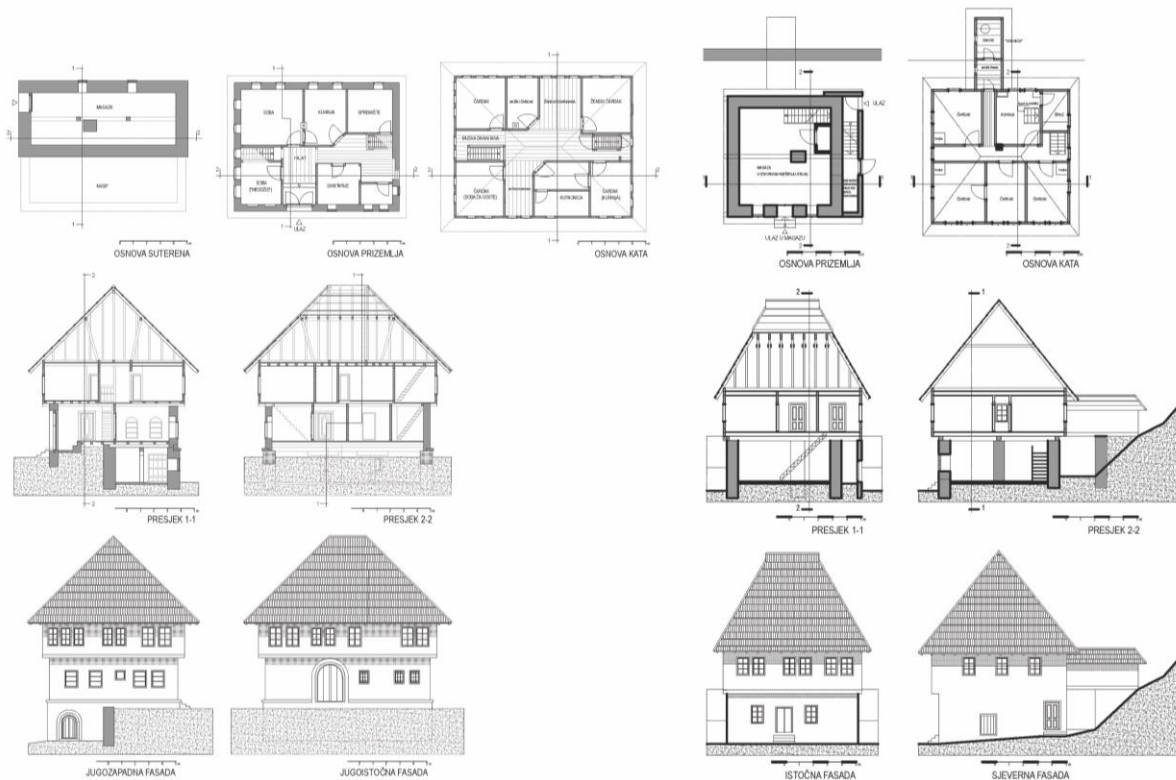
Figure 5. Drawings of the Pozderac (left) and Alagić (right) family houses in Cazin (Hadrovic, 2017)
