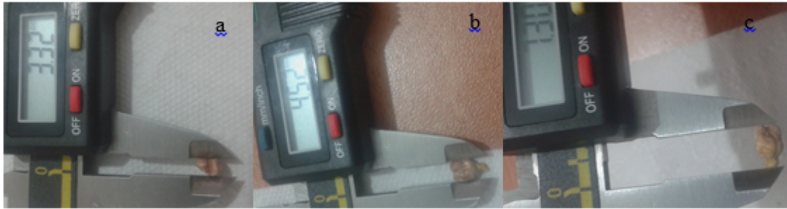
Figure 1. Method of measuring grape seeds a) method of measuring the thickness of the seed, b) method of measuring the width of the seed, c) method of measuring the length of the seed.
