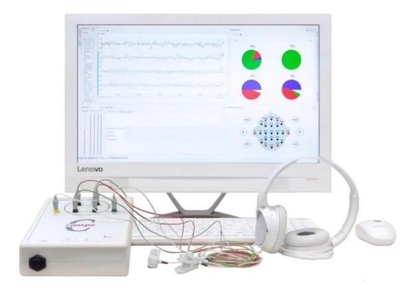
**Fig.1** Hardware complex "Synchro-C»: a device for converting the total electrical activity of the brain into the sound of the musical range for the bioacoustic normalization of the psychophysiological state of a person.
