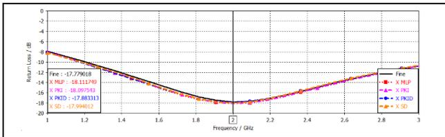
Figure 19. S-parameters produced by simulating ANNs results compared with fine,  $f_{opt}=2$  GHz.
