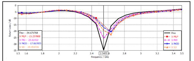
Figure 9. S-parameters produced by simulating ANNs results compared with fine,  $f_{opt}=2.54$  GHz.
