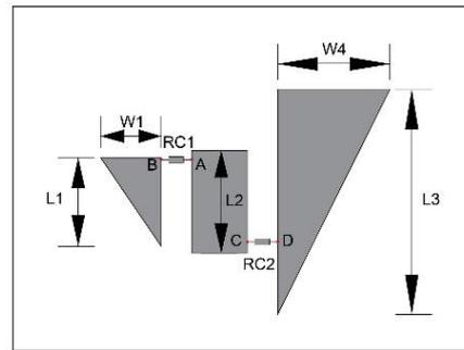
Figure 8. Production of a new model of RNSMA by using parameters of  $X_{MLP}$ ,  $f_{opt}=2.54$  GHz.
