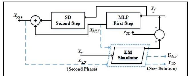
Figure 5. Hybrid structure including SD modeling in the second training step.
