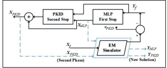
Figure 7. Hybrid structure including PKID modeling in the second training step.
