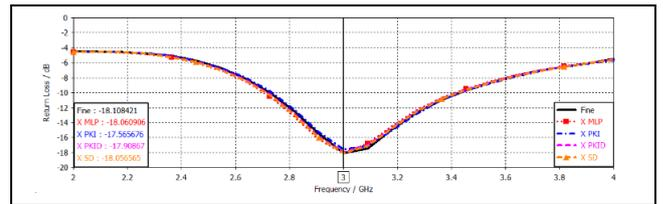
Figure 15. S-parameters produced by simulating ANNs results compared with fine,  $f_{opt}=3$  GHz.
