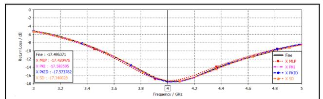
Figure 17. S-parameters produced by simulating ANNs results compared with fine,  $f_{opt}=4$  GHz.
