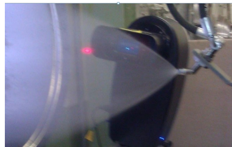
Figure 4: Spray Particle analyzer system
