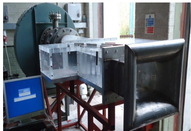
Figure 5: Suction wind tunnel compressor Cascade
