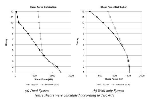
Figure 2: Shear Force Distribution along the Wall Height
