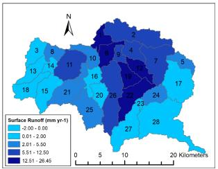
Fig. 7 Difference (LANDSAT 7 ETM model - Corine Model) map of the annual surface runoff (mm yr<sup>-1</sup>) calculated based on the simulation period (2010-2013)
