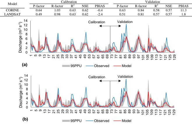
Fig. 5 Hydrographs at discharge stations representing observed data and model simulations, as well as the uncertainty in 95PPU (grey color) outputs of (a) CORINE Model, (b) LANDSAT 7 ETM Model
