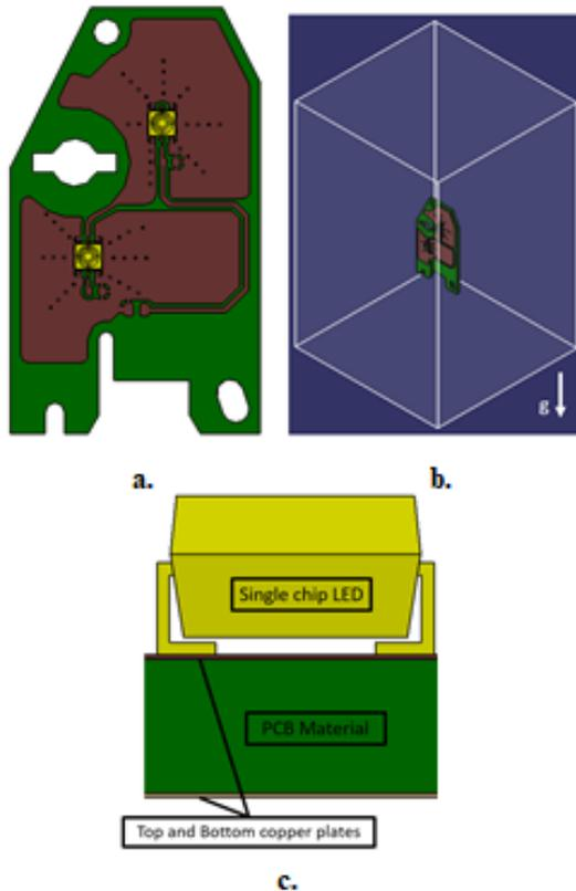
Figure 1: a. PCB with single-chip LEDs
