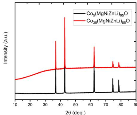
Figure 1. XRD patterns of the as-synthesized  $\text{Co}_5(\text{MgNiZnLi})_{95}\text{O}$  and  $\text{Co}_{35}(\text{MgNiZnLi})_{65}\text{O}$  HEOs.
