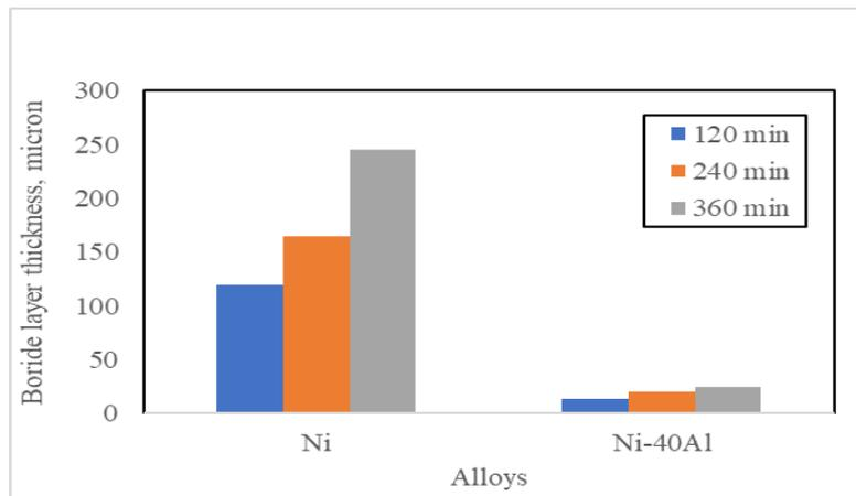
Figure 3. Boride layer thicknesses of the borided samples
