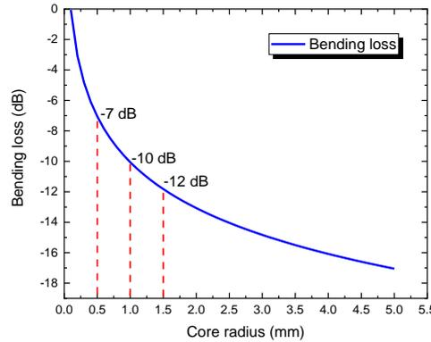
**Figure 2.** Bending loss versus fiber core radius
