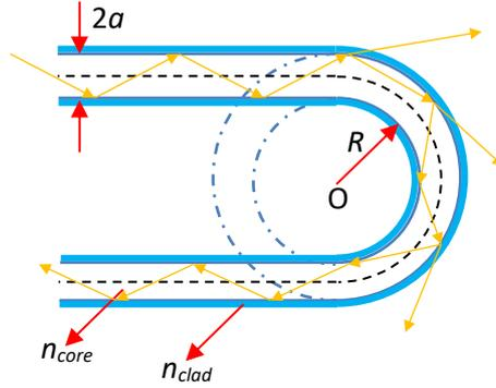
**Figure 1.** Losses in fiber due to bending effect
