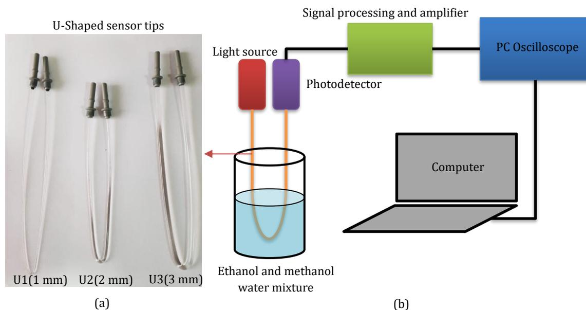
**Figure 3.** (a) U-Shaped sensor tips, (b) The block diagram of the experimental setup
