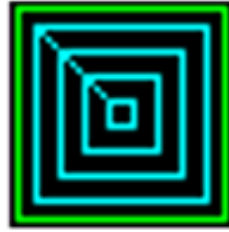
Figure 9: Parallel spiral toolpath strategy
