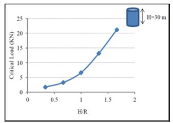
Figure 7. Variation of critical load versus h/r of tank h=30 m.
