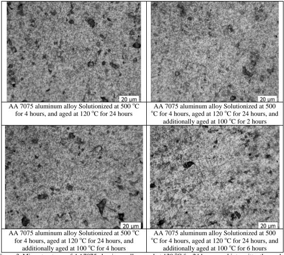
Figure 3. Microstructures of AA7075 aluminum alloy aged at 120 °C for 24 hours, and intermittently aged at 100 °C for 2, 4, and 6 hours.
