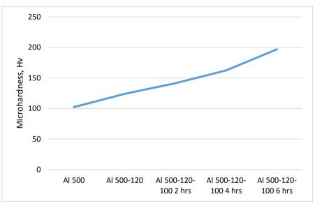
Figure 2. Microhardness change versus aging heat treatment
