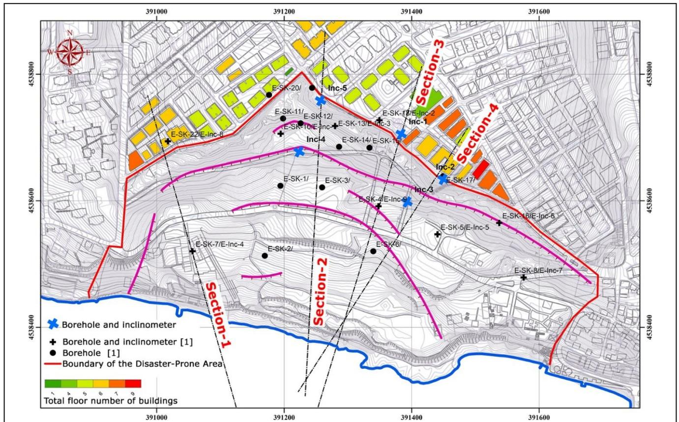
Figure 1. Borehole and inclinometer measurement points, section lines, surface ruptures of landslide in the study area (modified from Güler et al. [1]) and total floor number of buildings in the impact area.
