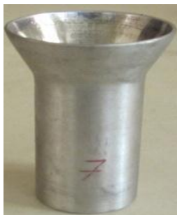
Fig.3 Expansion of tube with the die of r_p/r_0=1.53 , \alpha=30^\circ
