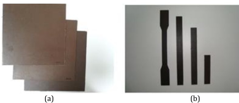
Fig. 3 (a) Produced bark flour filled composites, (b) Test samples
