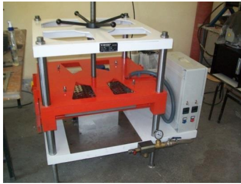
Fig. 1 Thermoforming unit used in experiments
