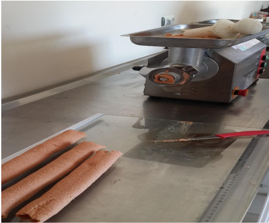
Figure 3. Cylindrically shaped outer shell passing through stuffed meatballs apparatus.
