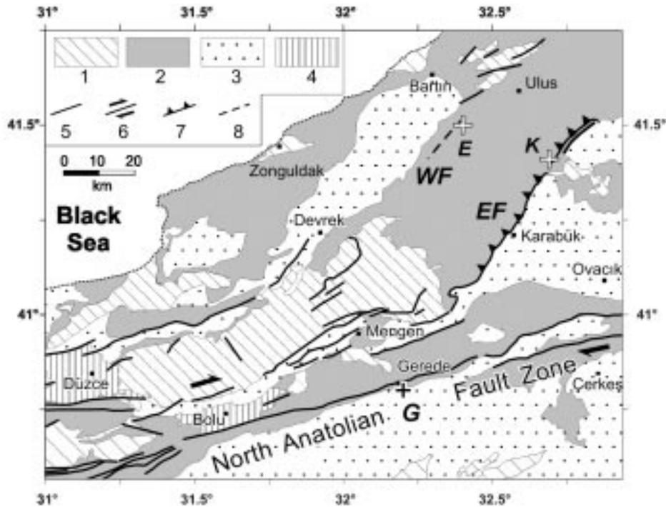
Figure 2. Simplified geological map of the area studied (Key to legend. 1: Paleozoic units; 2: Mesozoic units; 3: Tertiary units; 4: Quaternary basin deposits; 5: Fault; 6: Strike-slip fault; 7: Thrust fault; 8: Probable fault. Geological data from 1/500.000 scaled geological map (Zonguldak Sheet, MTA) and Tüysüz (1993). E, G, and K: epicenter locations for the 1944 earthquake. EF (Eastern fault) and WF (Western fault) are two fracture zones discussed in text).
