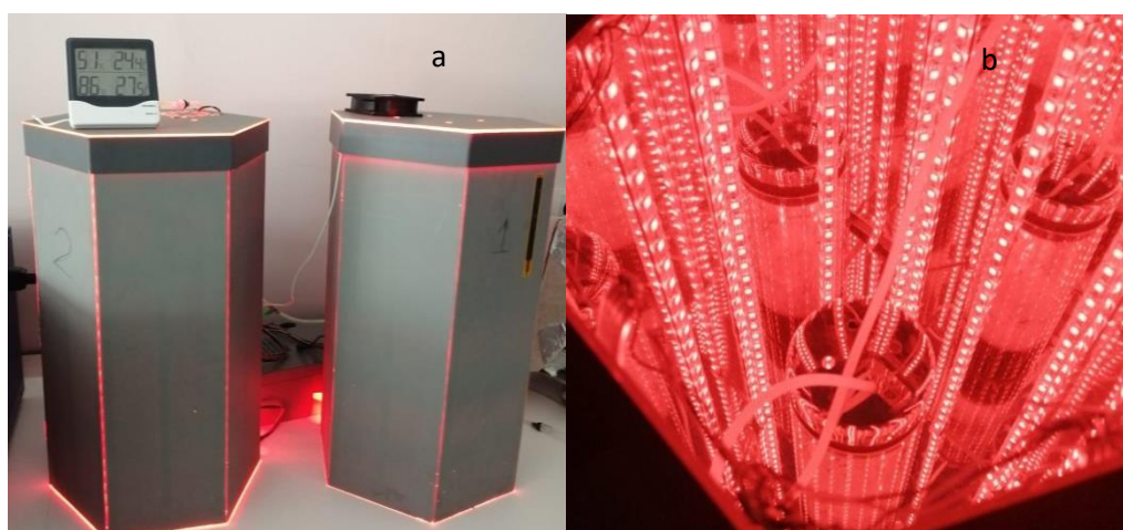
Figure 2. The designed photobioreactors a) outer view b) interior view under red light.
