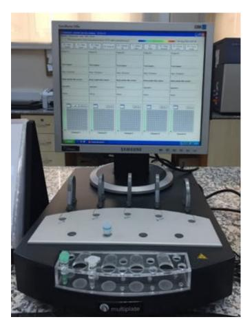
Fig. 1. Multiplate Test Machine. Multiplate test machine in our hospital is located in Hematology laboratary; however, it is possible to be situated and utilized it with a trained staff in interventional radiology units.
