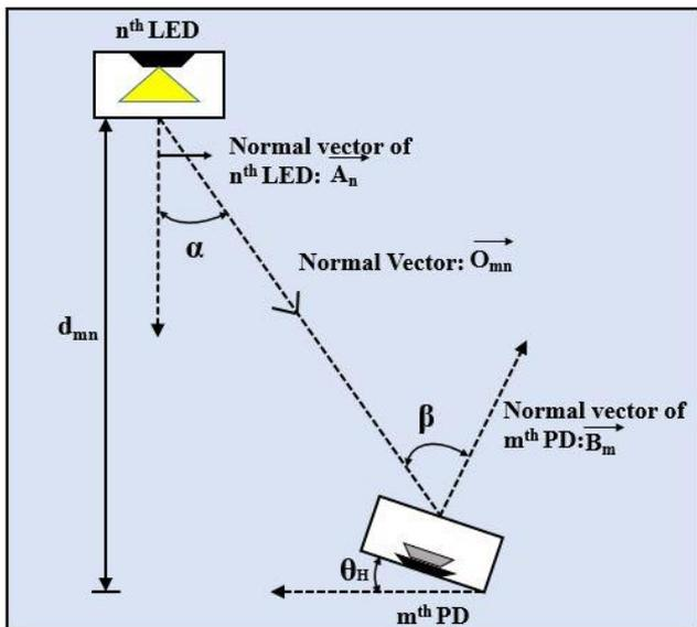
Figure 2 The geometry of LED-PD pair
