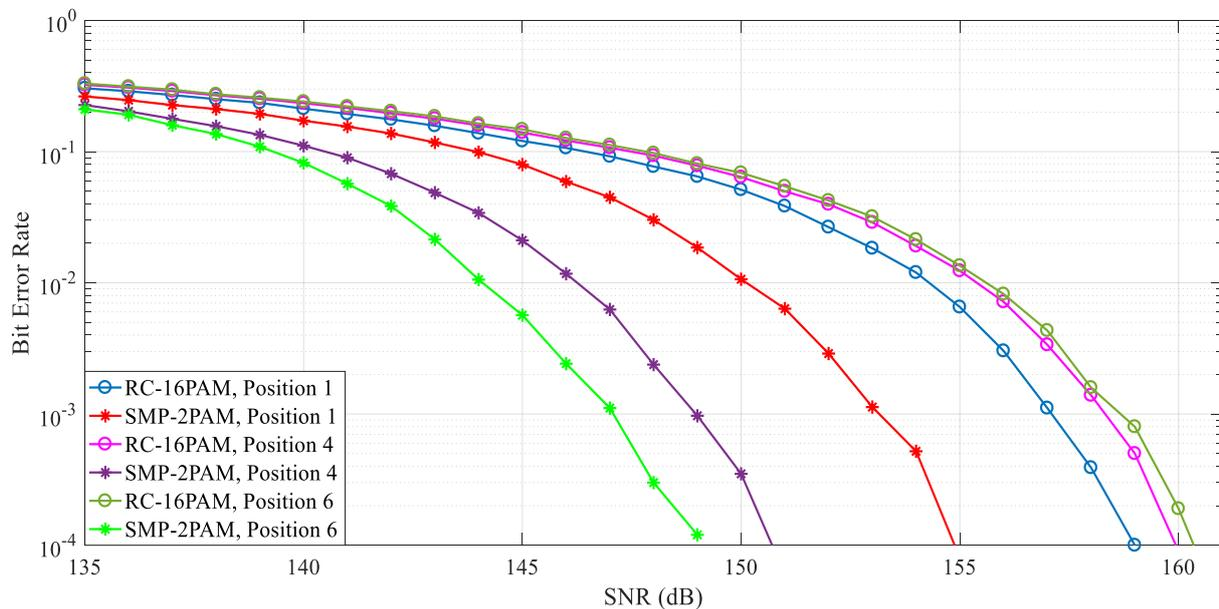
Figure 12 BER performance comparison of RC and SMP
